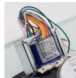
70/25V transformer with colored leads
